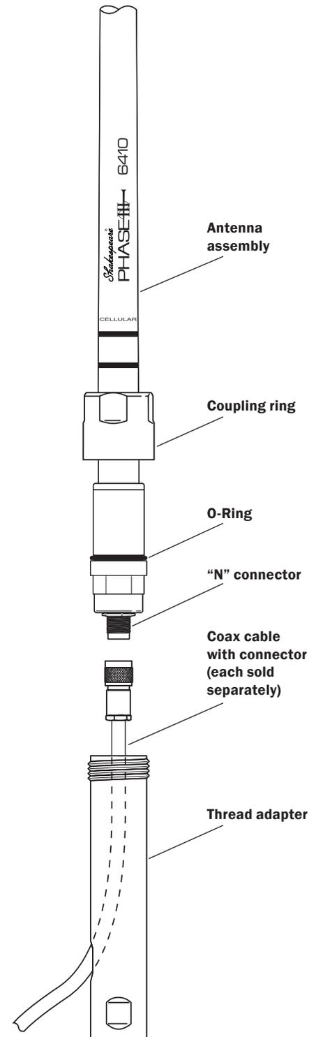
3. Attach the “N” connector to the base of the antenna and tighten securely.
