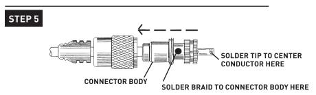
Screw the connector body tightly onto the reducing adapter and solder the tip to the center conductor. Trim off any excess center conductor. Solder the braid to the connector body through the holes. Screw the coupling ring on, and slide the DooDad® Cable Strain Relief snugly onto the rear of the completed connector.
