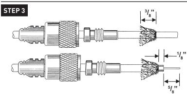
Fan the braid back, as illustrated, and trim it to 3/8". Strip the insulation from the center conductor as shown. **Be careful not to damage the center conductor.**
