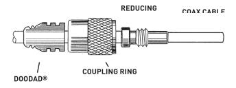
**Separate all parts to individual components.** Slide DooDad®, coupling ring, and reducing adapter onto the cable in the order and orientation shown.
